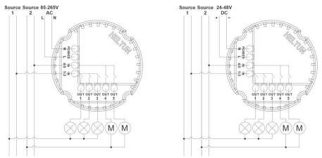
Figure 2: Connection Diagrams
